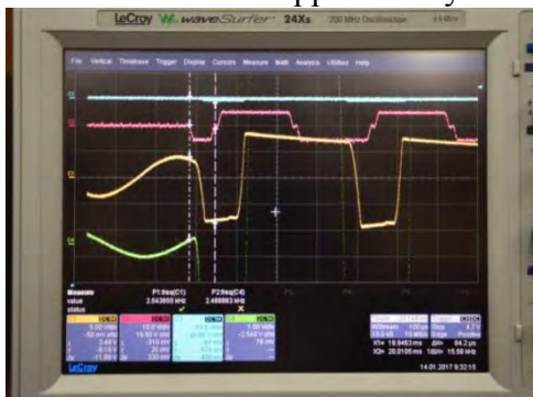
Fig. 16. Adjustment of the suppression in the quadrature channel by changing the duration and phase of the first suppression pulse
