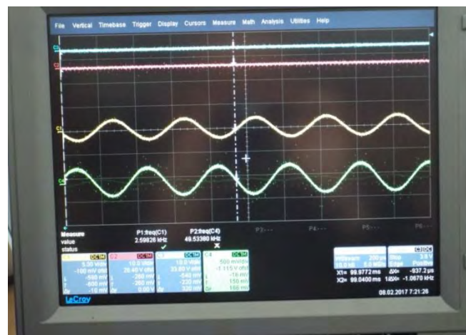
Fig. 19. Rotate the gyroscope clockwise. Rotation speed 10 degrees per second
