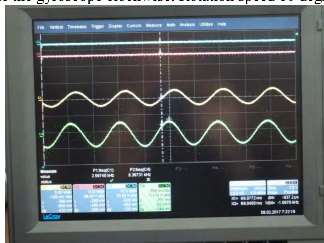
Fig.20. Rotate the gyroscope counter clockwise. Rotation speed 10 degrees per second. The change in the phase of the oscillations in quadrature channel carries information about the direction of rotation
